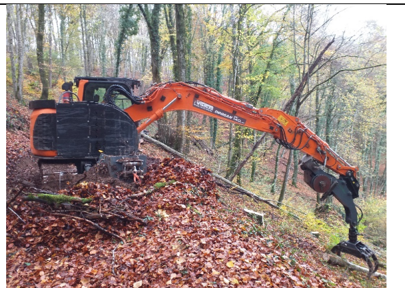
Figure 6: When the grapple is used, the multifunction hub is stuck under the boom
