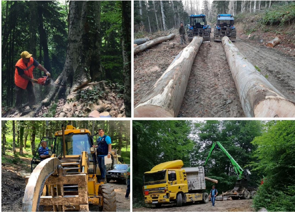
Figure 4. Motor-manual tree felling, tractor skidding and hydraulic operated crane assisted timber loading
