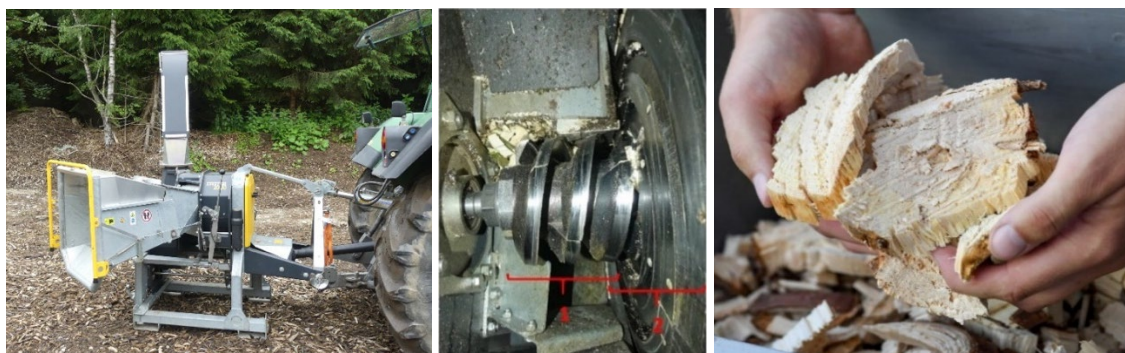
Figure 1: left: The Effiter 20.30 duplex-spiral chipper powered by a conventional farm machine; middle: Duplex spiral of the Effiter 20.30 with the cylindrical screw on the left (1) and the flat screw on the right (2) as seen from the inspection hatch; right: Effits from stemwood of Norway spruce (photo: Tobias Hase, StMELF)
