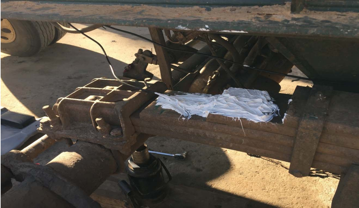
Figure 3: Strain gauge coated in protective caulk.
