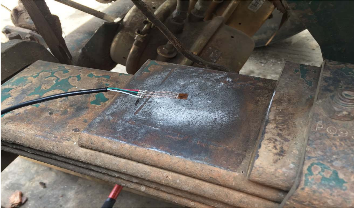
Figure 2: Strain gauge adhered to leaf spring.
