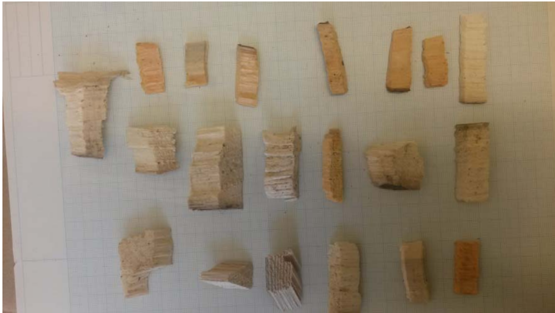
Figure 2. Examples of chips in the 16-31.5 mm class. Each large square = 10×10 mm, subdivisions 1 mm
