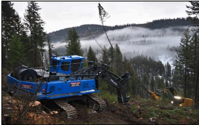
Figure 5. Falcon winch-assist and Tigercat LX870D: Case Study 5
