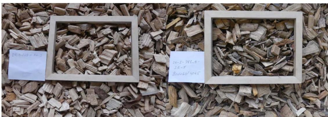
Figure 6: Left: Reference wood chips (stemwood of Norway spruce) after processing in supply chain I (size of the rectangular frame = DIN A5). Right: Roadside maintenance wood chips upgraded in supply chain I (size of the rectangular frame = DIN A5)
