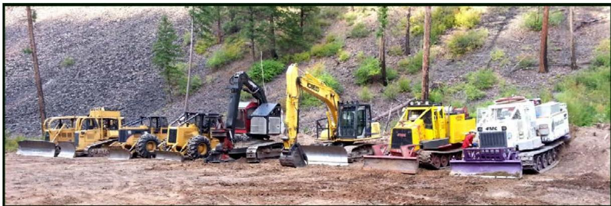
*Image 2 - Left to Right: Dozer, pumpercat, wheel skidder, wheel skidder with drop-tank, feller-buncher, excavator, softtrack skidgines*
