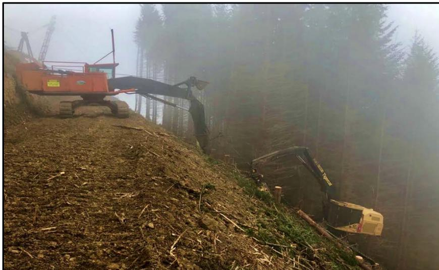
Figure 1. Waka Welding Ltd winch-assist and Tigercat LS855D: Case Study 1
