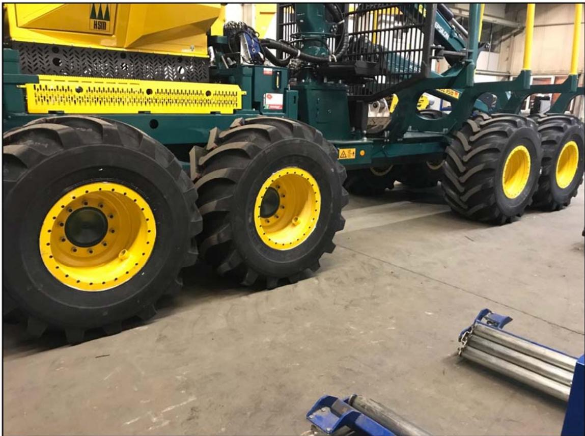
**Fig 7: Test forwarder with bead-lock rims**
