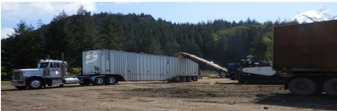
Figure 1. Grinder feeding a highway tractor with hog fuels. These trucks are often restricted by volume and not weight depending on the states they operate.
