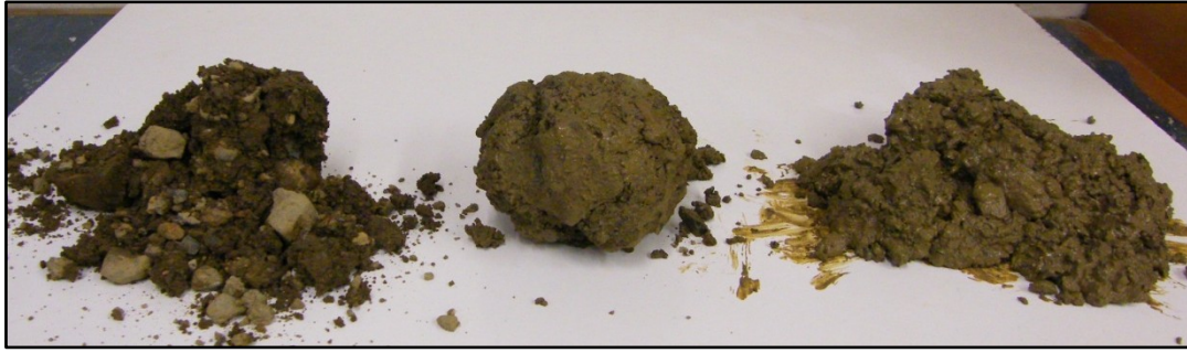
Figure 2: A photograph showing the method used to determine OMC. The samples on the left and right are too dry and too wet respectively. The middle sample has been prepared at OMC.
