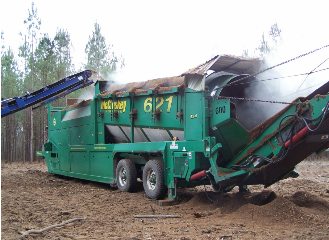
Figure 1: A trommel screen receiving grindings from a horizontal grinder in a planted pine stand in South Carolina, January 2011.
