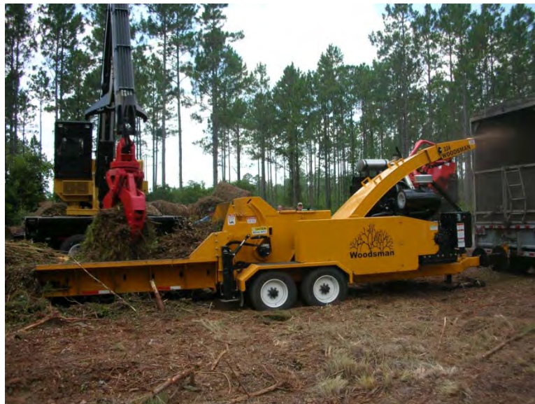
Figure 1. Processing bales with a Woodsman 334 horizontal drum chipper.
