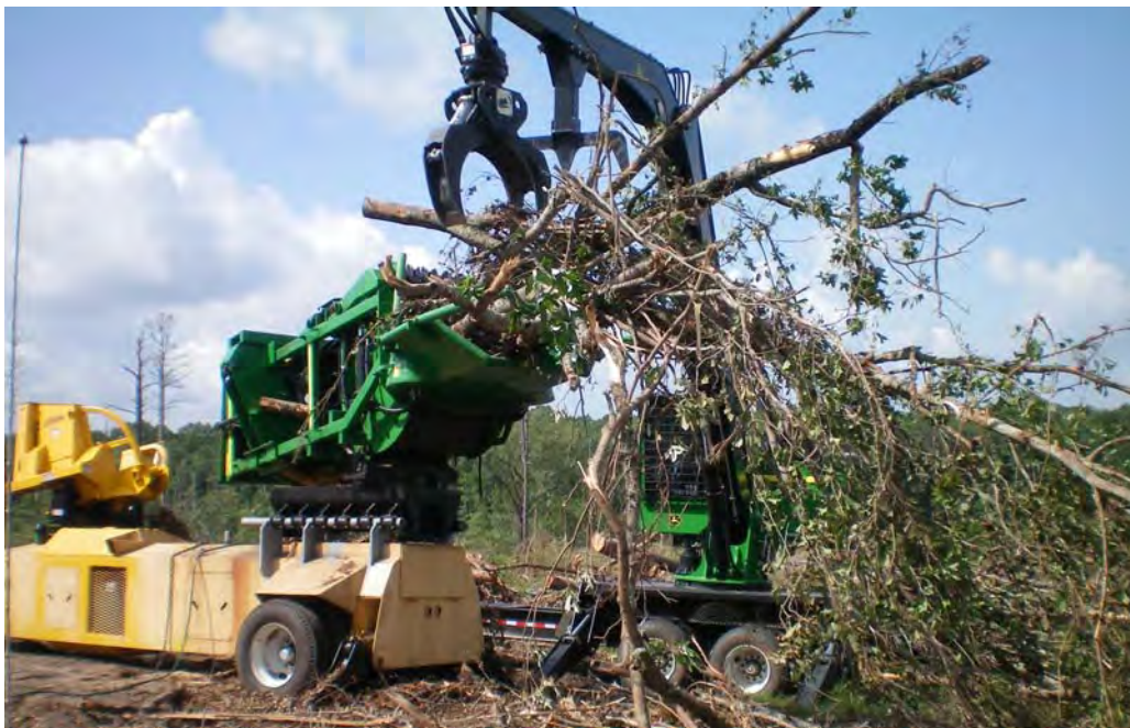
Figure 3. Bundling hardwood slash at the Midway test site.
