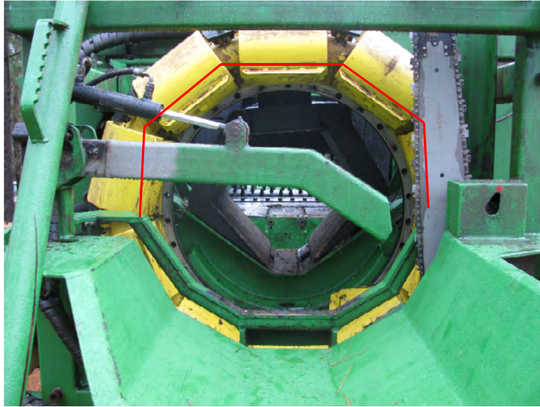
Figure 6. Location of the hold down bar protection.
