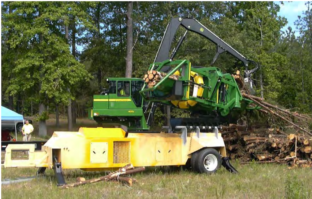
Figure 2. Initial testing of the bundler in Auburn, Alabama.
