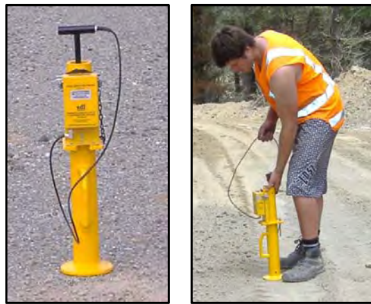
Figures 1a and 1b: The Clegg Impact Soil Tester (left) and the CIST being used to test the subgrade of an East Cape forest road (right).
