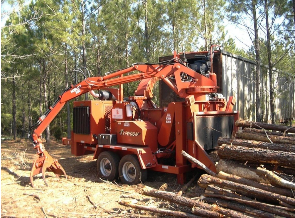
Figure 3. Morbark Typhoon chipper with a loader attachment.
