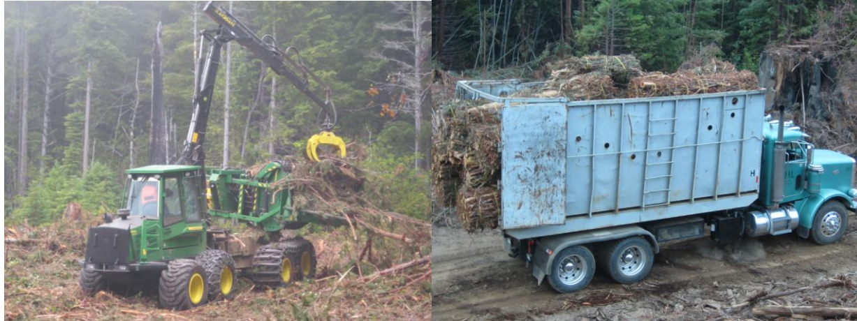
Figure 2: John Deere 1490D energy wood harvester which produces the bundles, and hook-lift truck used to haul bundles.
