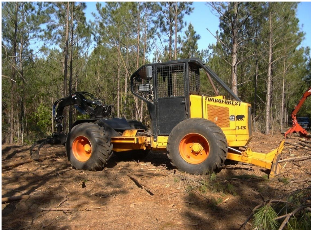
Figure 2. Turbo Forest skidder with a grapple attachment.
