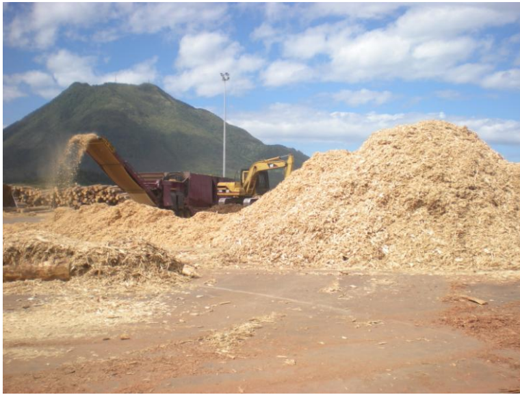
Figure 2: Tub grinder working at the CPY in Kawerau. This CPY processes over 500,000 m 3 of wood annually
