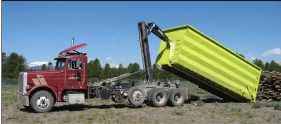
Figure 1: Hook-lift truck unloading a roll-off bin of slash at the concentration site used in the Hebgen Lake study
