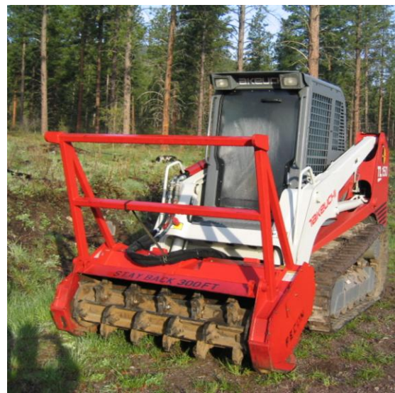
Figure 2. Horizontal drum masticators: boom mounted (left) and integrated (right).
