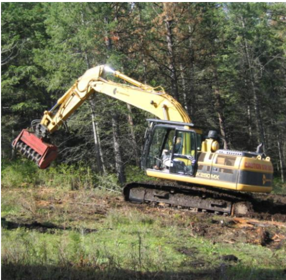
Figure 2. Horizontal drum masticators: boom mounted (left) and integrated (right).
