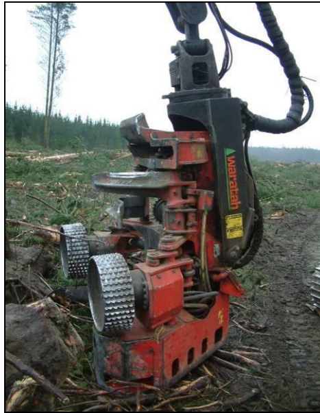
Figure 2: The Waratah 622 harvesting head in Bottlelake Forest.
