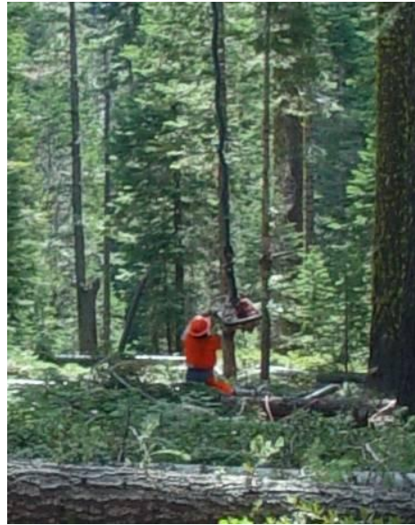
Figure 2: A hooker putting the chokers onto the hook.
