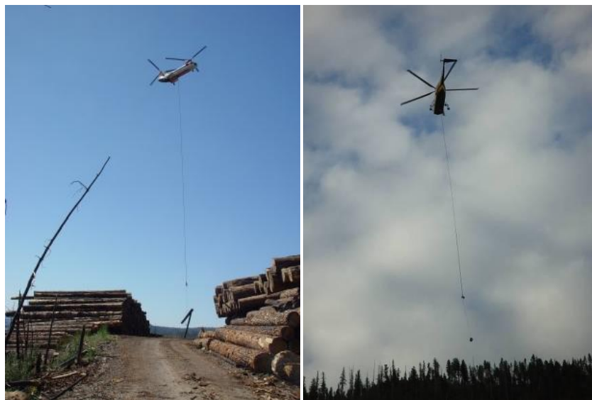
Figure 3. Left: Helicopter at the drop zone (unhooking), and right, helicopter with chokers going to woods (outhaul).
