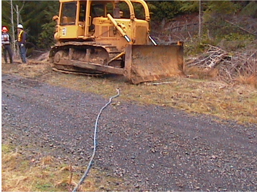
Figure 4. Synthetic rope skyline extension (7/8-inch by 200 foot AmSteel® Blue) laid out from the tailhold Cat into the unit.
