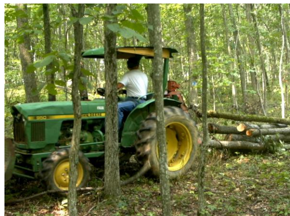
Figure 1. 4wd John Deere Tractor used for extraction
