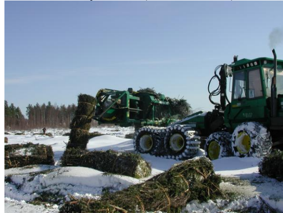
Figure 1. Composite residue logs produced by Fiberpac slash bundling technology. Courtesy of Dr. A. Timperi, Timberjack Oy, Finland.
