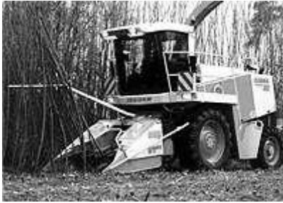
Figure 1. Claas forage harvester with HS-2 header (Source: www.claas.com)
