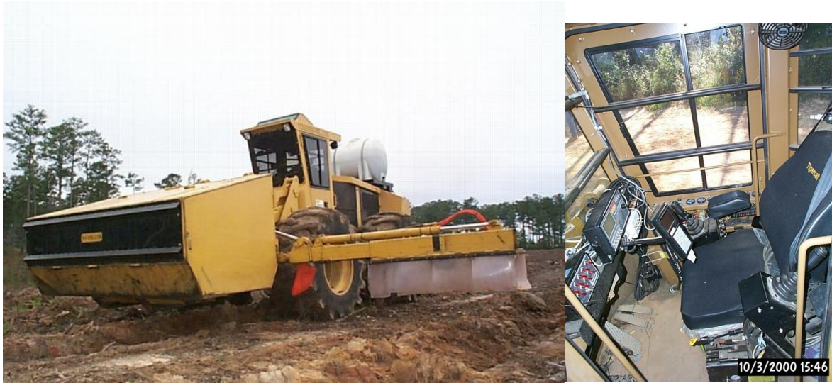
Figure 1. Photograph of WS sprayer configured for banded spraying. Inset shows the cab with field computer and other spray controller equipment.
