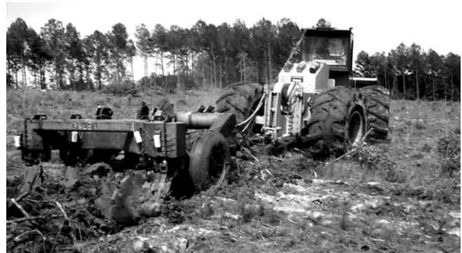
Figure 1. Supertrac SK-300 pulling a Savannah 310 trailing subsoil plow with coulter, ripping shank, and four disks
