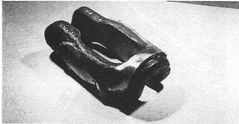
Figure 3. An aluminum shield bonded over the strain gages and wires
