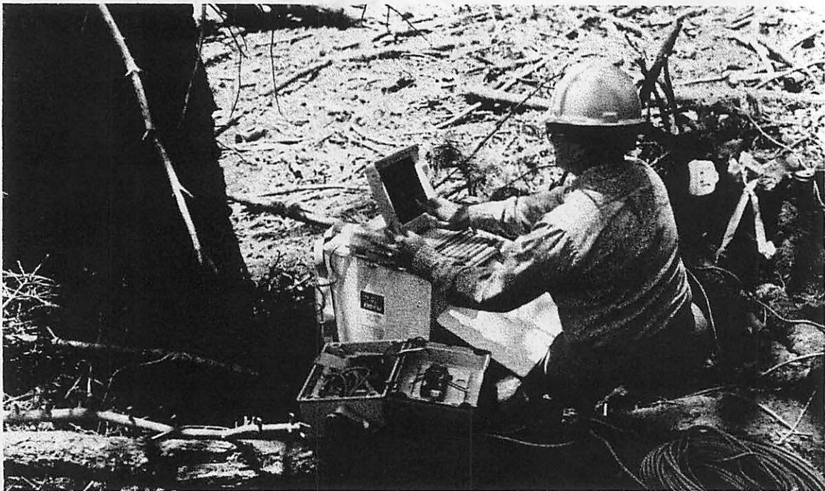
Figure 6. The CR10 and Data General One at use monitoring guyline loads.
