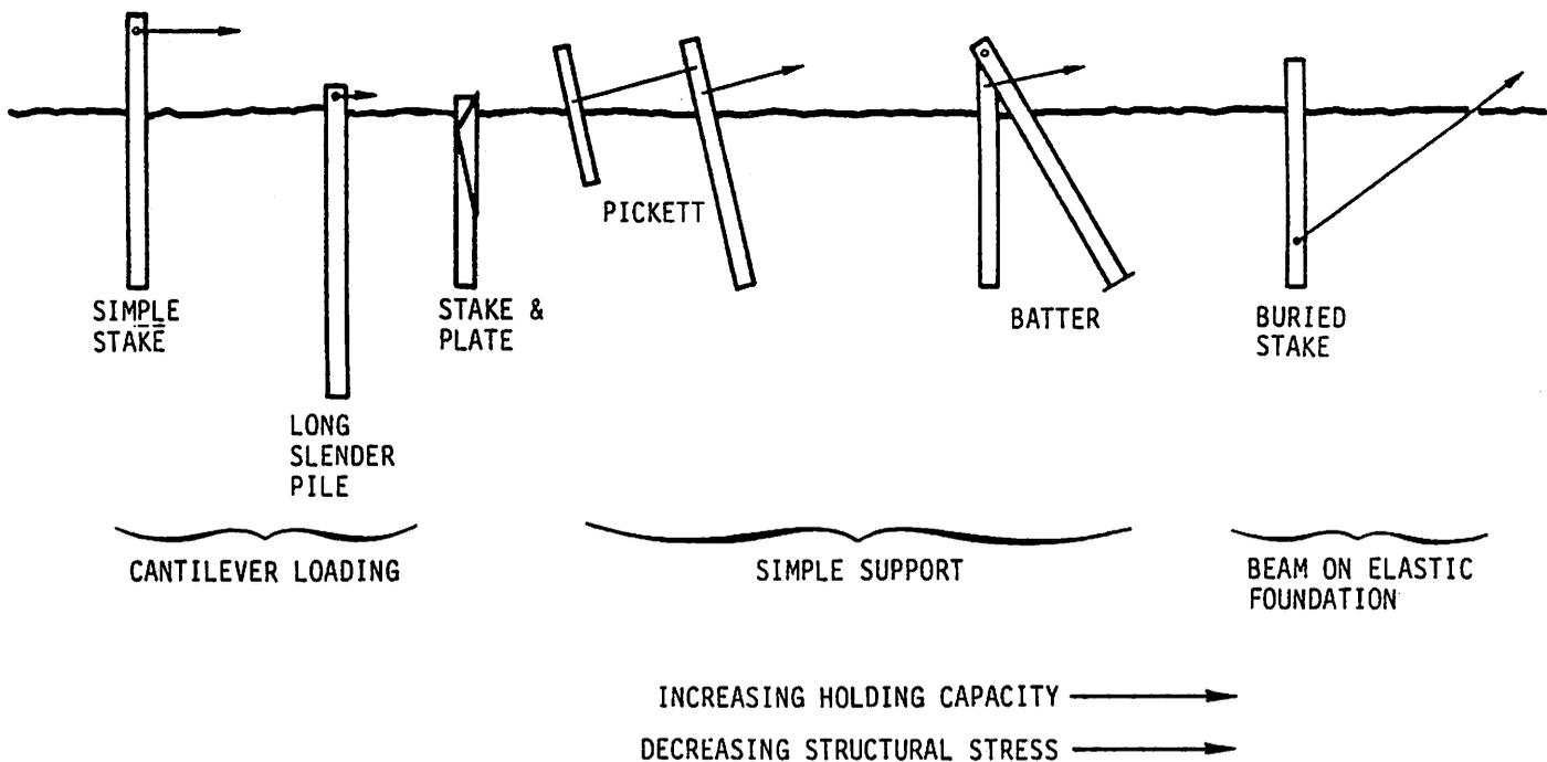
Figure 3.--Laterally loaded pile anchors.
