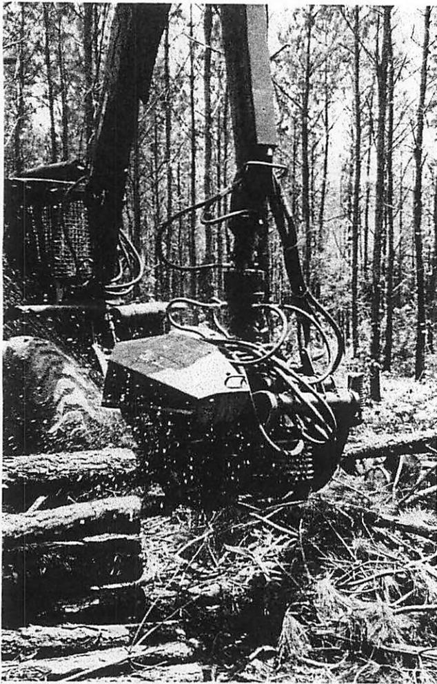
Figure 1.--The Valmet 940 GP grapple processor.
