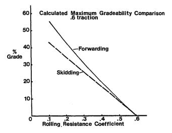
Since we would like to move the product from stump to roadside with a minimum of energy expended, the load is carried on rubber-tired wheels rather than allowed to partly drag on the ground. The numbers are clearly favourable when making comparisons with grapple skidders.
