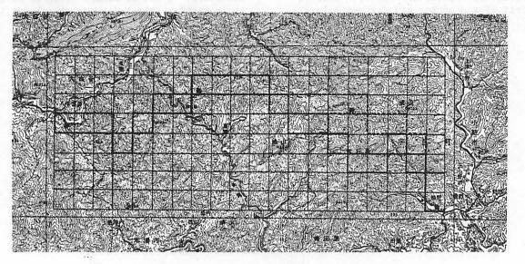
Figure 4.--Contour map overlaped with the series of grids showing the best route for the forest road.
