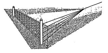
Figure 6.--Soil-net anchor concept.
