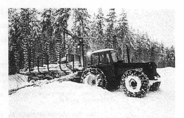
Figure 2. Modern Valmet 802 farm tractor equipped for forwarding wood
