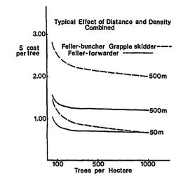
A good way to examine the economics of this sequential multi-function machine is to look at it separately, first, as a feller-buncher, and then, as a selfloading forwarder. The machinery provided can be identified as: that for felling only; that for forwarding only; and that which works at both.
