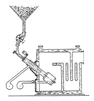
Figure 2.--Pellets burner with rotation combustion basket.
