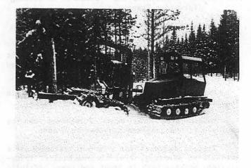
Figure 7. Farmi-Track is a modern tracted forwarder for thinnings
