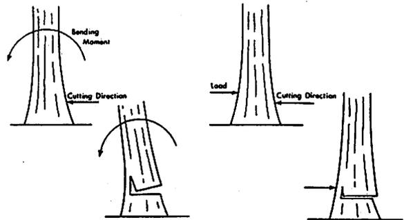
Figure 4.--Bending moment and/or loads perpendicular to the tree during the cutting phase result in butt damage.
