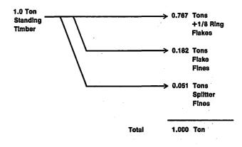
Figure 9. Material Balance for Producing Ring Flakes From Chunks From One Ton of Standing Timber O.D. (Oven-Dry) Basis.
