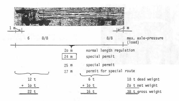
Figure 4: Loading capacities and transport regulations for timber transport
