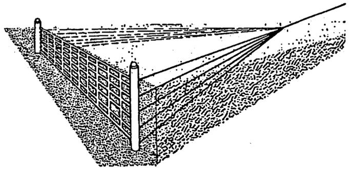
Figure 6.--Soil-net anchor concept.
