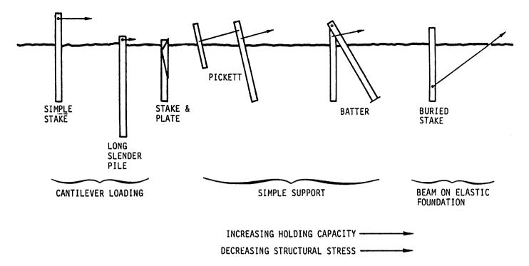
Figure 3.--Laterally loaded pile anchors.
