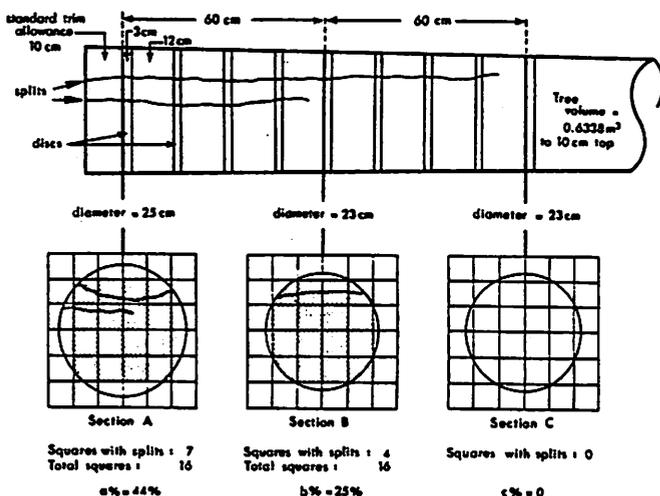
Figure 2.--How to measure butt damage using the bicycle-wheel method. The technique was so named because the first grid developed consisted of a rim from a bicycle wheel strung like a tennis racket.
