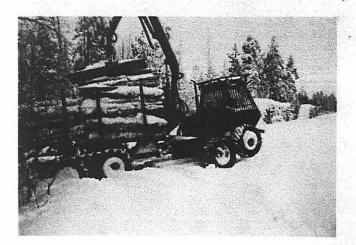
Figure 9. Forwarders of the future will be lighter and smaller. Norcar is one example of them
