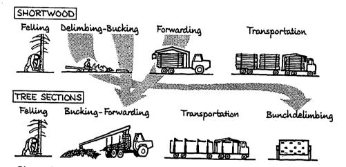
Figure 1. The logging system strongly influences the design of the transportation system.
