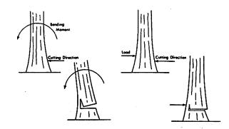
Figure 4.--Bending moment and/or loads perpendicular to the tree during the cutting phase result in butt damage.
