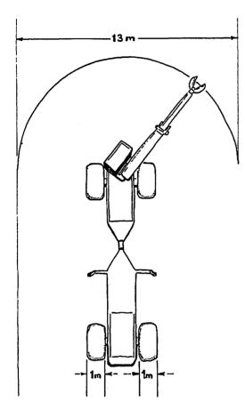
The feller-forwarder, with its longreach boom and easily controlled travel, is mechanically suitable for thinning and sorting operations. Calculations indicate that there will be little productivity loss if at least 200 trees per hectare are taken, and provided the remaining trees are in straight strips, or number 150 or less per hectare.
