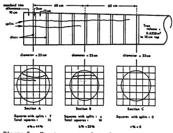
Figure 2.--How to measure butt damage using the bicycle-wheel method. The technique was so named because the first grid developed consisted of a rim from a bicycle wheel strung like a tennis racket.
