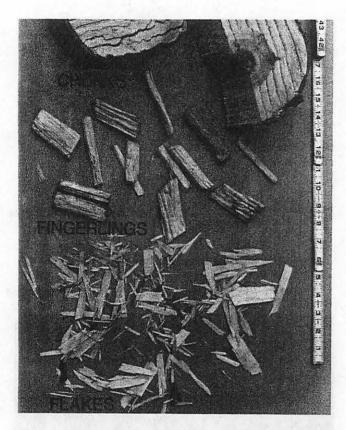
Figure 6.-- Aspen Chunks Produced by the Forest Service Involuted Disc Chunking Machine, Fingerlings That Were Split From Chunks in the Institute of Wood Research Prototype Chunkwood Splitter and Ring Flakes Made From the Fingerlings.
