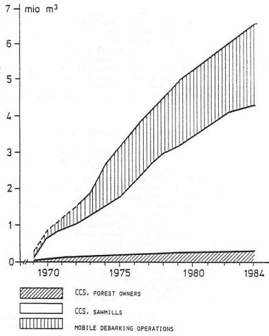
Figure 2. Mechanized debarking at central coversion site and at roadside in the Federal Republic of Germany.
