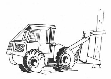
Figure 1.--Typical feller-buncher with chassismounted shear.
