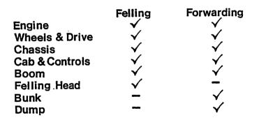
As we get into this, we see that there is very little that does not work at both operations; and, even then, the temporarily extraneous components or abilities are sometimes of advantage. For example, the bunk would not be needed if bunches were built on the ground, but, particularly in sparse stands, it assists felling in that the operator always has a place to put his trees.
