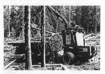
Figure 4. Modern Bruunett mini 572 forwarder is equipped with double boggies
