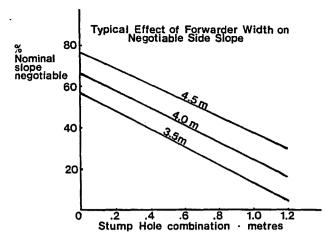
Tailoring wheel base to tree height, reference to stump hole combinations, machine width, and experience are all important in making side slope applications. Of course, just like any other stump area logging machine, feller-forwarders need to be designed to quickly go back to work after taking a tumble.
