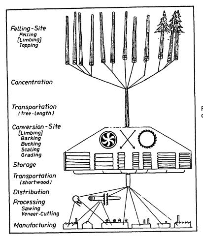
Figure 3. System of centralized and mechanized conversion.
