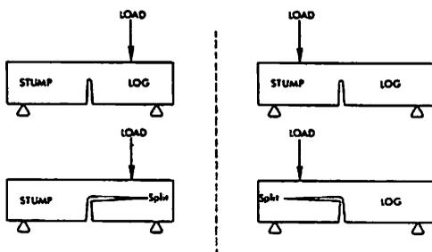
Figure 5.--The direction of splitting depends on how the load is applied to open the kerf.
