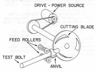
Figure 3.--Diagram of USFS Chunker
