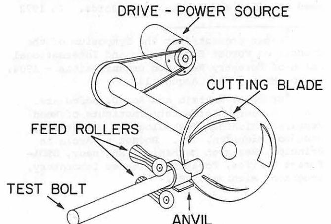
Figure 3.--Diagram of USFS Chunker
