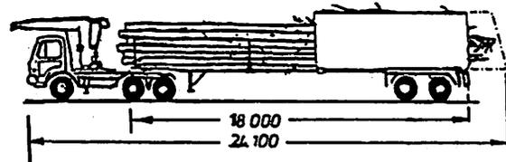
Fulltree-transport with semitrailer and steel box. The length of the trailer can be altered according to the size of the trees being carried.
