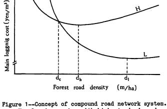
H : logging system with high standard roads and long span cable yarding. L : logging system with low standard roads and short span cable yarding.  $q = (p - d_0) \cdot d_0 + (2500 V \cdot (1+\eta) \cdot (\alpha_H \cdot (1+\eta'_H)))$
