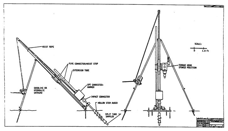
Figure 2.--Proposed soil testing and anchor installation apparatus.
