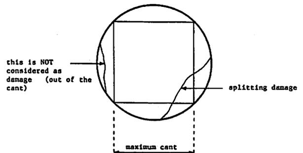
Figure 1.--Splitting damage as measured by the square-cant method.
