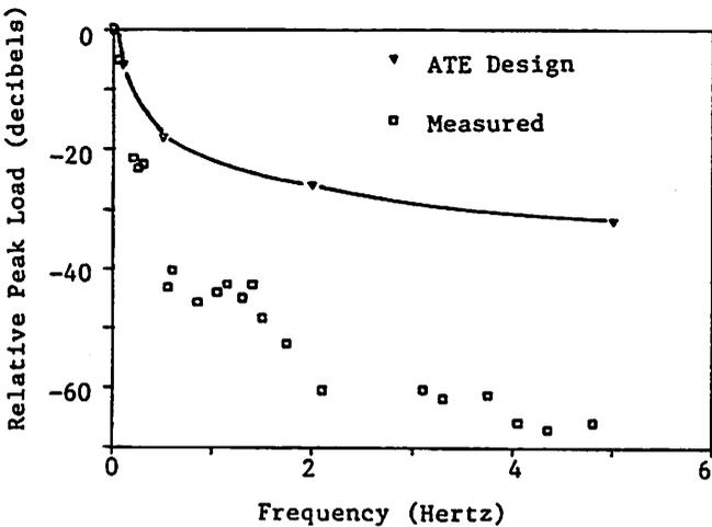
Figure 1.--Measured guyline dynamic loads and anchor testing equipment (ATE) design dynamic loads versus frequency.
