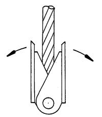
Figure 5.--Hinge-plate anchor.
