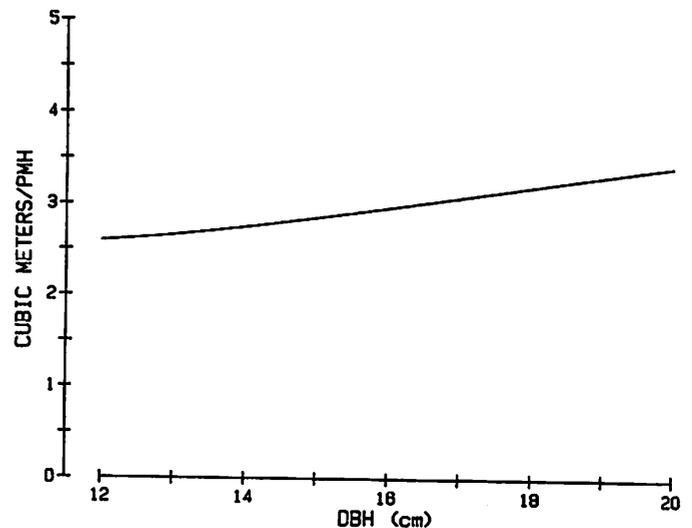
Figure 4.--Production rate as a function of DBH.
