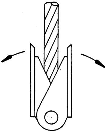
Figure 5.--Hinge-plate anchor.
