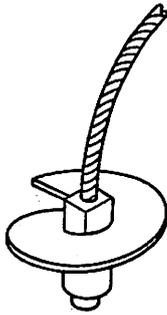
Figure 4.--Flexible connections for plate anchors minimize alignment requirements.
