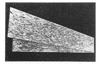
Figure 7.--Typical 1/2 x 16 x 96 Inch Panels Made From Chunked Wood.
