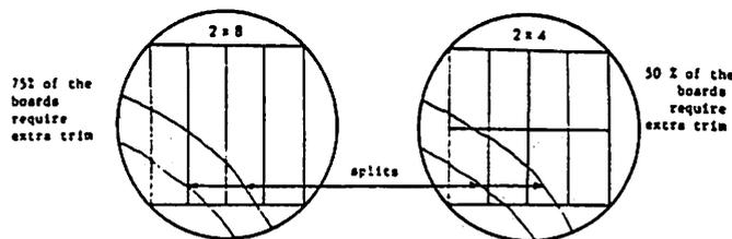
Figure 3.--Influence of the size of board cut on the percentage of wood loss.
