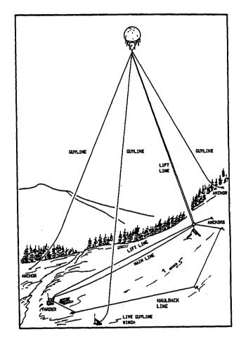
Figure 1.--Pendulum swing balloon logging systems.
