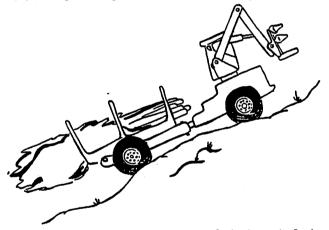
Side slopes are more detrimental to feller-forwarder operation and, for oscillated chassis configurations, what can be handled depends on roughness and how well the machine balance is arranged in the fore and aft direction.
