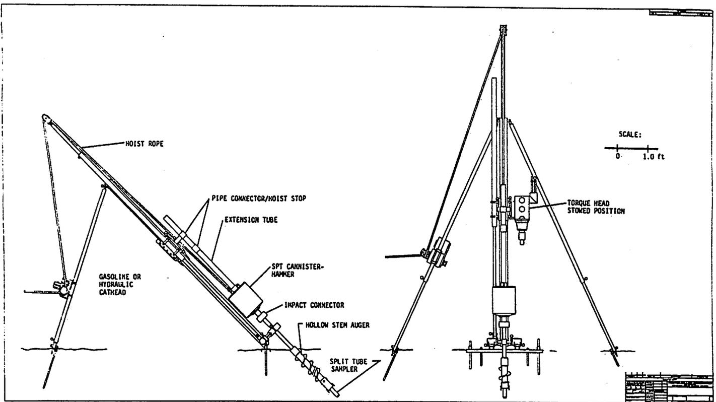
Figure 2.--Proposed soil testing and anchor installation apparatus.
