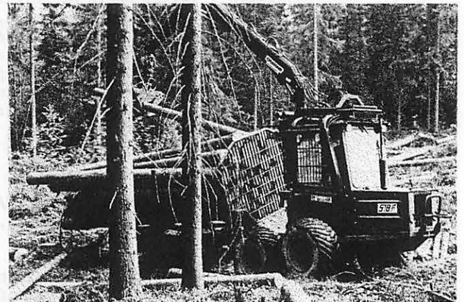
Figure 4. Modern Bruunett mini 572 forwarder is equipped with double boggies
