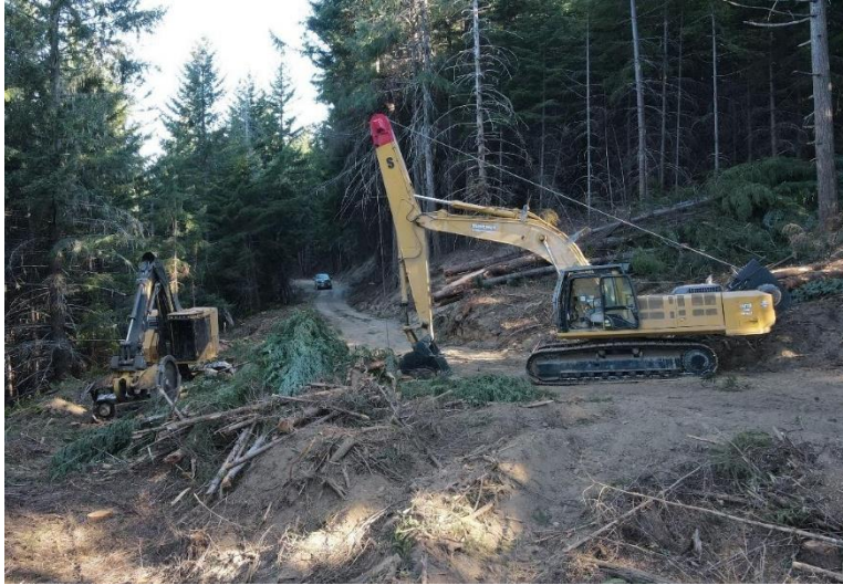
Figure 2. The Tigercat LX830D (left) tethered to the excavator-based Summit Winch-assist machine (right) at the ridge of Unit A.
