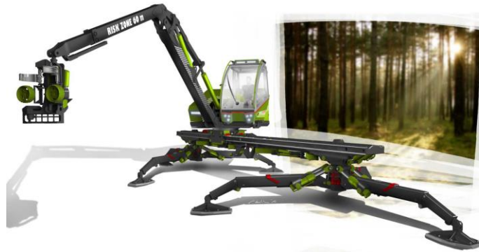
Figure 6. Representation of the portal advancing mechanism with a harvester crane. (Knobloch, 2017)
