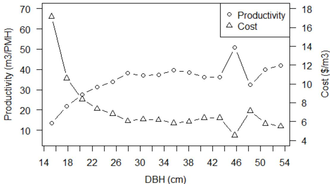
Figure 1. Predicted productivity ( $\text{m}^3/\text{PMH}$ ) and cost ( $\$/\text{m}^3$ ) of the harvester relate with tree size in DBH (cm)
