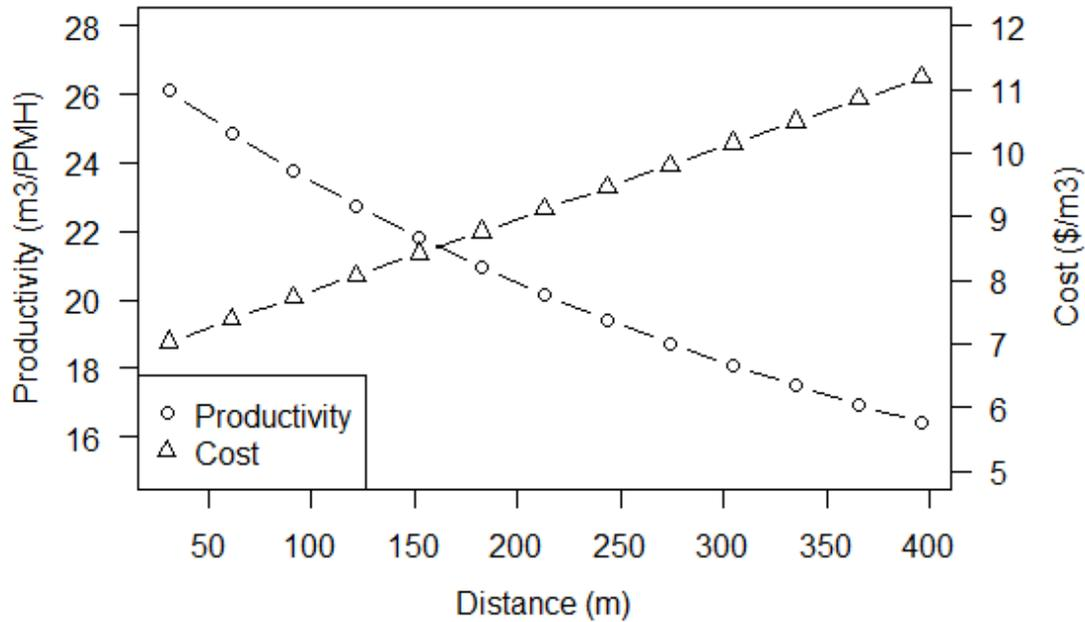
Figure 2. Predicted productivity (m<sup>3</sup>/PMH<sup>a</sup>) and cost (\$/m<sup>3</sup>) of the forwarder relate with loaded moving distance (m)
